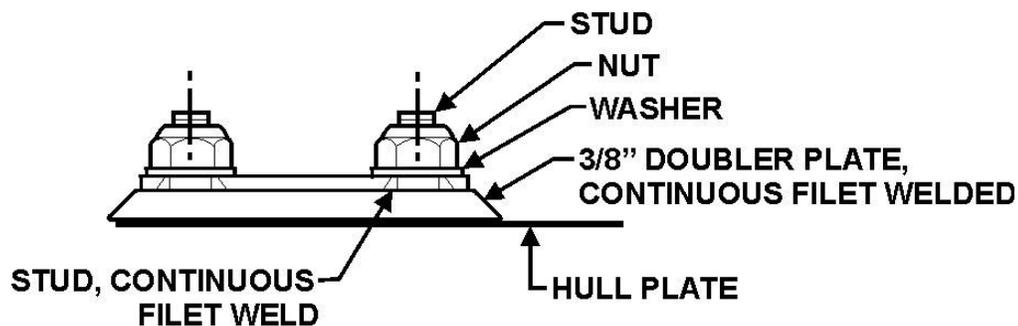
**Figure 1-1. Zinc Anode Stud and Doubler Plate Attachment**
