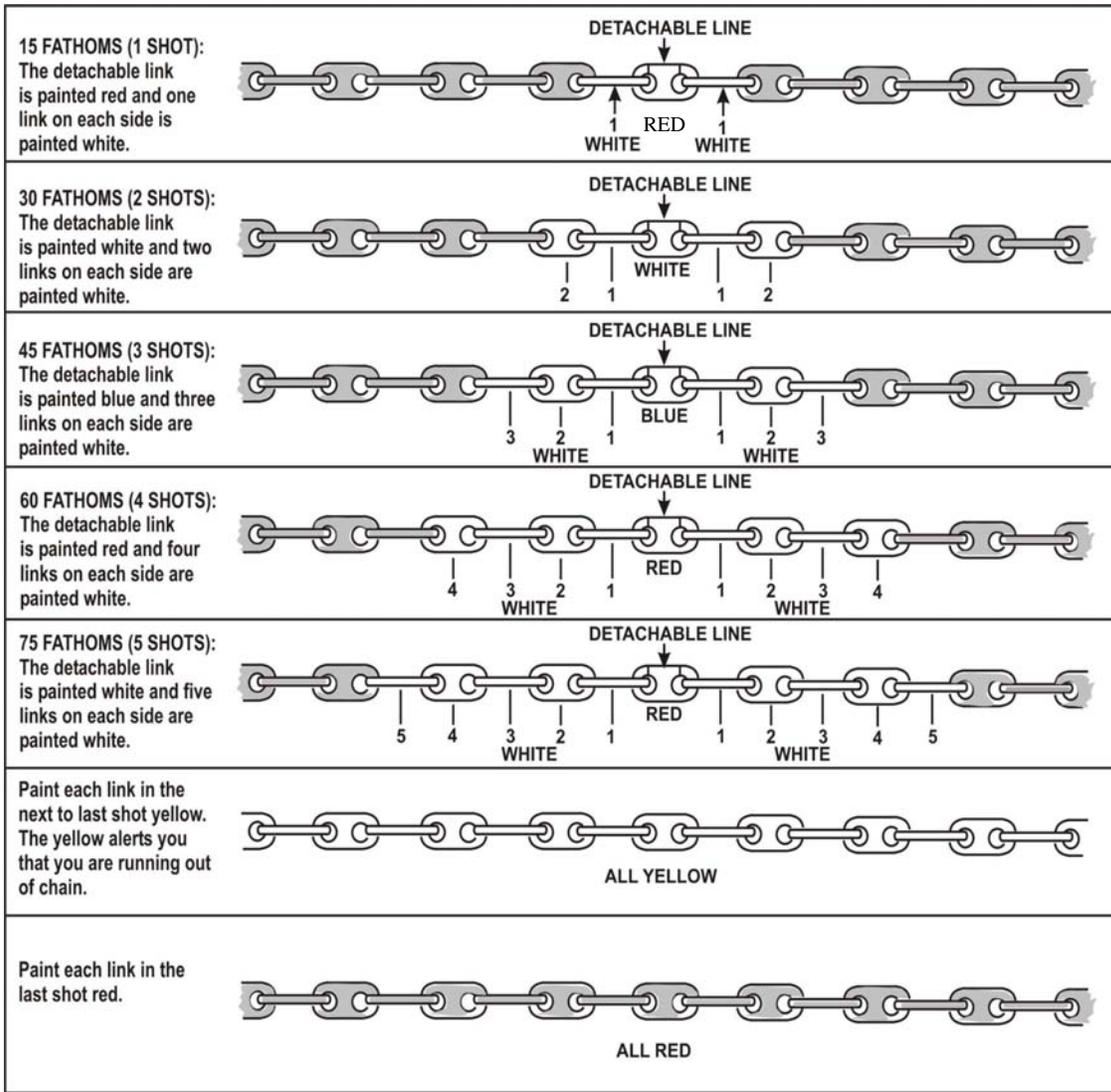
**Figure C-1. Standard Anchor Chain Markings.**
